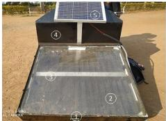
Figure 1. Experimental set up of front side of Hybrid type of Solar dryer. 1. DC blower at inlet of collector, 2. Absorbing plate, 3. Baffle 4. Drying Chamber, 5. Solar Panel
