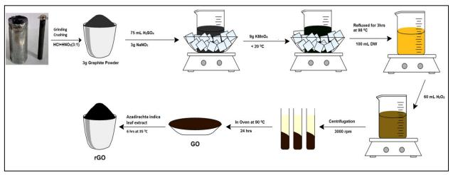
Figure. 1. Systematic procedure of synthesis of GO and rGO from graphite powder obtained from waste battery cells.
