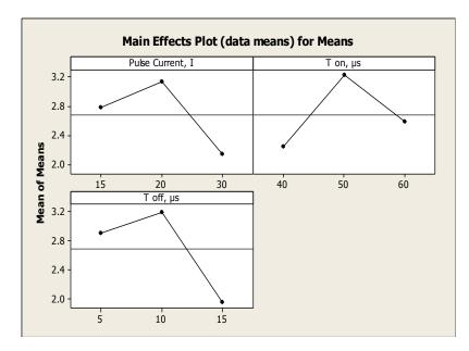
Fig. 2. Main Effect Plot (Copper Electrode)
